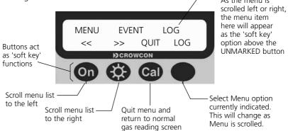
The four buttons have above them a symbol or word: these are the 'soft key' functions currently assigned to that particular key. Use the ON and BACKLIGHT buttons to scroll left and right, the CAL button to quit the menu system and the UNMARKED button to select a menu option. View the road map on page 37 for details of Detective+ configuration menu system
