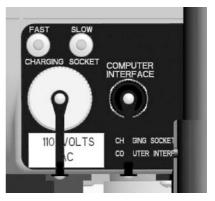
UNDER NO CIRCUMSTANCES MUST THE COVER BE REMOVED OR THE CHARGING LEAD BE CONNECTED TO THE UNIT WHEN IT IS LOCATED IN A HAZARDOUS AREA.
